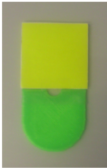
Figure 4.8: Close-up of the two-colour marker. The green colour is used for localization purposes while the yellow one is employed to compute robot's orientation.
