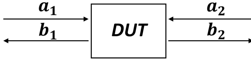
Fig. 2.9.2. A representation of S-parameters for two port device under testing.
