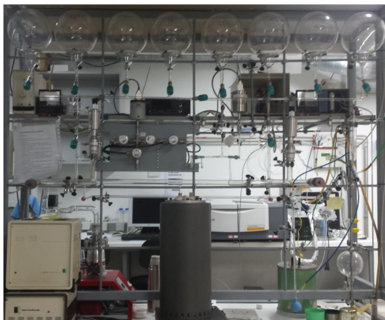
Volumetric equipment coupled to microcalorimeter.
