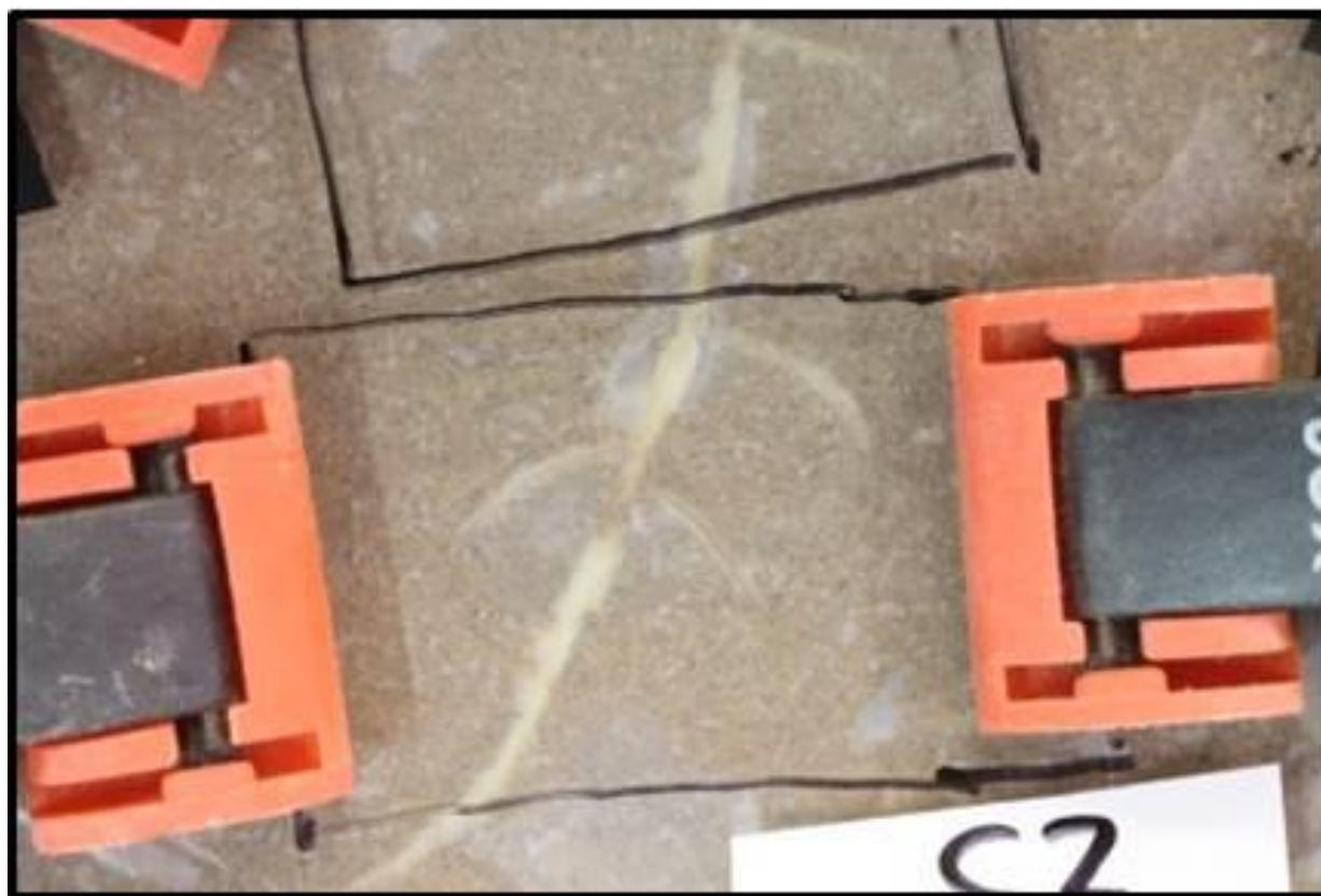
Figure A-5. Detail of gel deployment on a white lupin root. Clamps are used to make pressure on the front plate of the rhizotron to assure contact between the gel and the soil surface (the nucleopore membrane is between the soil and the gel).
