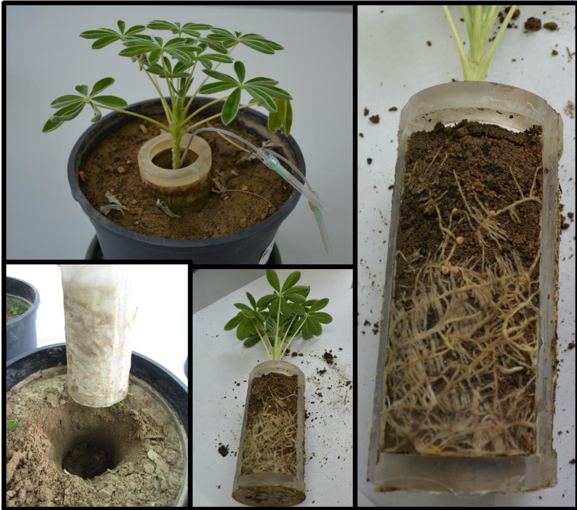
Figure A-3. Details of the rhizobag system and porewater collection described in Chapter 4.2.
