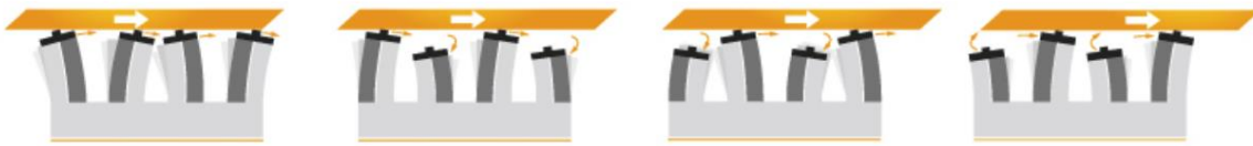
Figure 2.1 Principle of operation of the piezoelectric motors used in this PhD, Piezo LEGS® from PiezoMotor®. Source: http://www.piezomotor.com/
