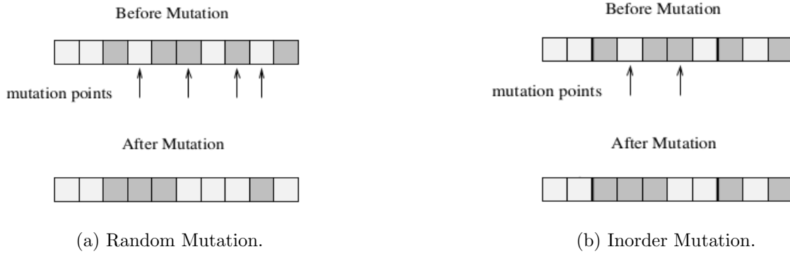
Figure 3.1: Mutation operators for binary representations.
