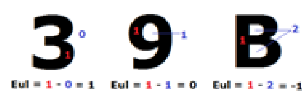
Figure 4.12: Calculation of the Euler number on different shapes
