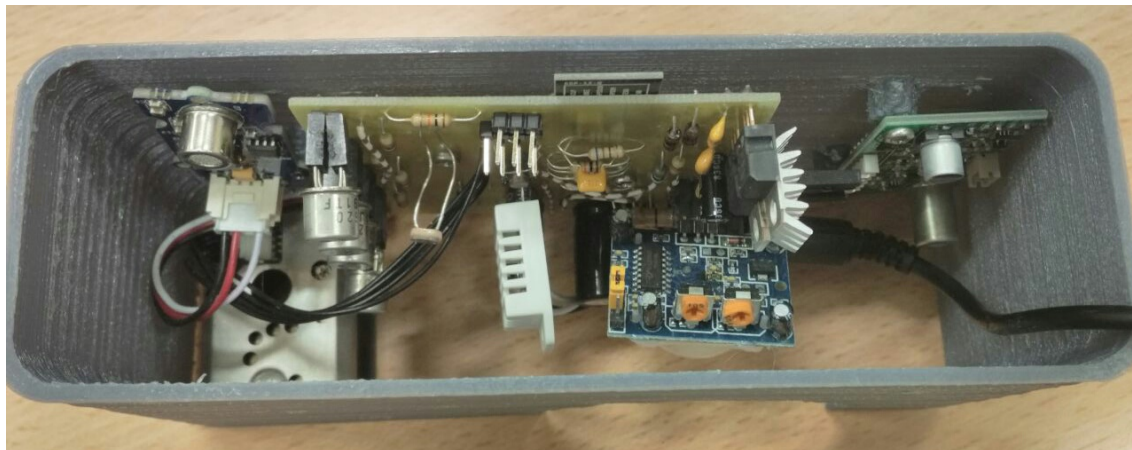
Figure 3.1: The e-nose installed in the classroom number 5.
