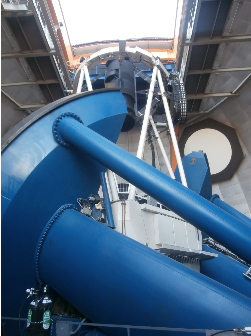
Figure 3.1: DECcam mounted at the focus of the Victor Blanco Telescope. Image credit: M. Garcia-Fernandez
