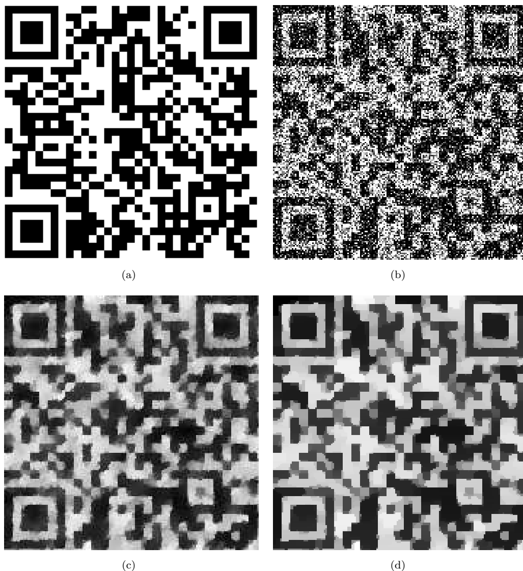
FIGURE 4.5: QR code image (a) Original image (b) Noisy image (c) Isotropic denoising (d) Anisotropic denoising.
