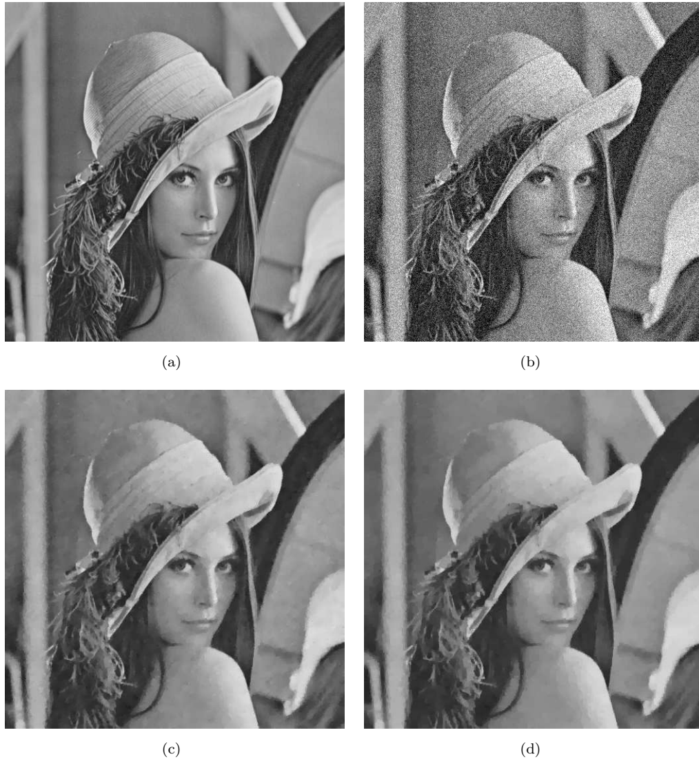
FIGURE 4.4: Lena image (a) Original image (b) Noisy image (c) Isotropic denoising (d) Anisotropic denoising.
