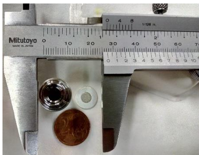
Fig. 19. Top view of Sieverts reactor and filter
