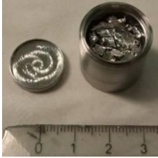
Fig.13. Open annealing sample holder. Adapted from [30]
