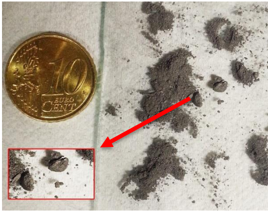
Fig. 68. Particles after hydrogenation experiment. Inset figure in red frame is a zoom of agglomerated particles
