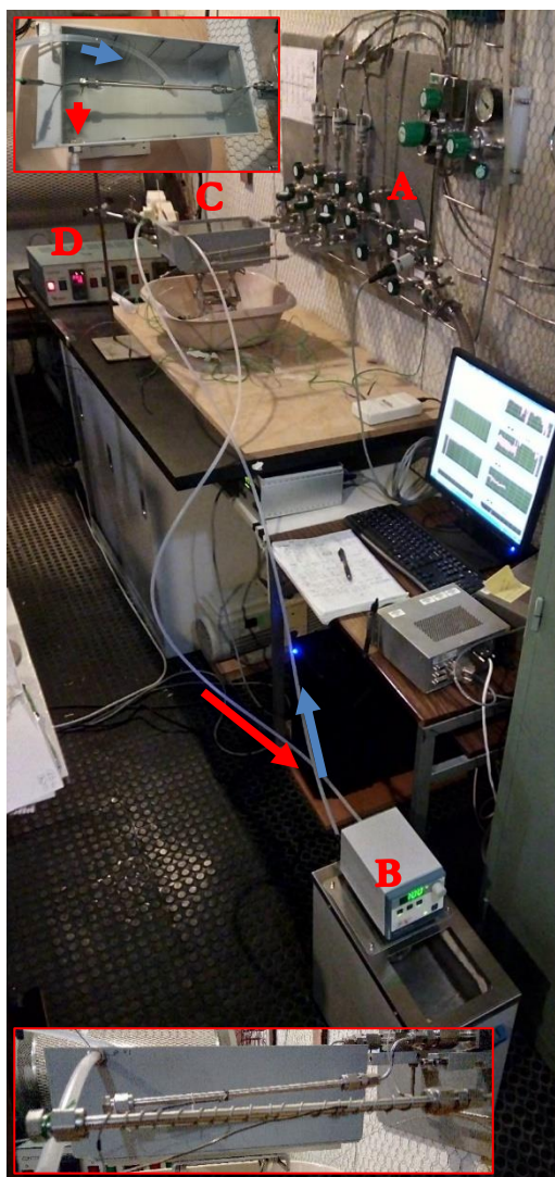
Fig.83. Complete MHHC test system, A. Sieverts-type MHHC test system, B. circulating bath system, C. Thermal bath vessel and D. heating control unit. Inset pictures are a zoom of the thermal bath (up) and the thermocoax surrounding the reactor (bottom)
