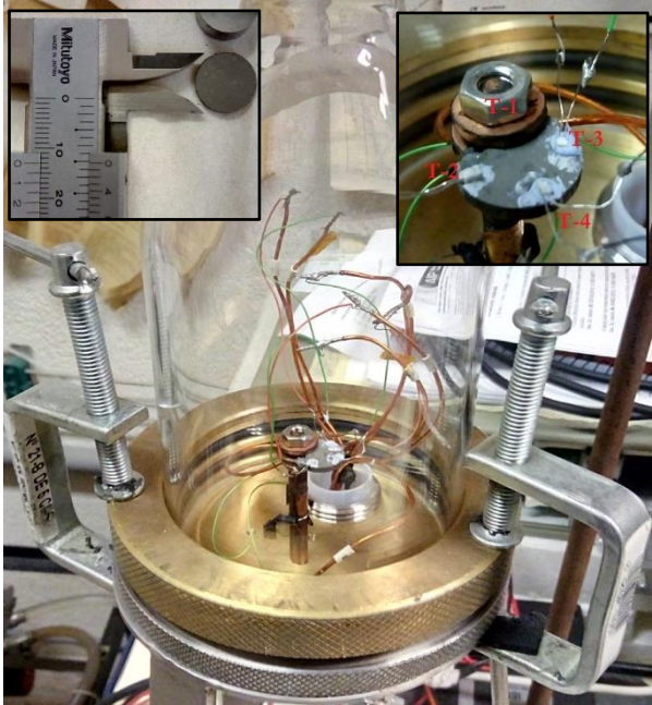
Fig.23. Thermal conductivity system. The inset picture of the left is the compressed sample, while the inset picture of the right is a zoom of the sample in the vacuum chamber with all the thermo-resistances (T-1, T-2, T-3, T-4)
