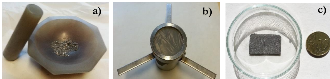
Fig.16. XRPD sample preparation, a) agate mortar and pestle, b) sieve of 45 \mu\text{m} , c) sample prepared on a quartz plate
