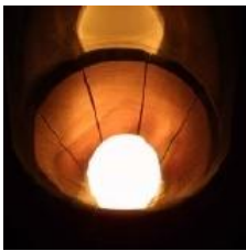
Fig.10. Synthesis by arc melting furnace. a) scheme of the system, b) fusion chamber
