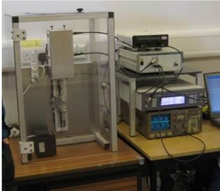
Figure 1.13. AC susceptometer at Institute for Science and Technology in Medicine, Keele University, UK. Reproduced with permission.
