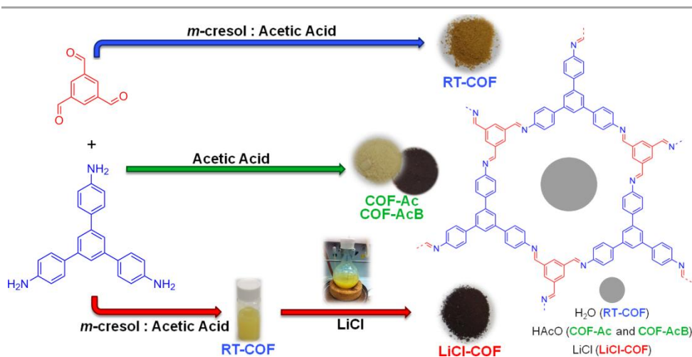
Figure 4.1. Schematic representation of the synthesis and structure of RT-COF (top), COF-Ac (middle) and LiCl-COF (bottom). The grey circle represents the guest molecules accommodated in the channels of the COFs.
