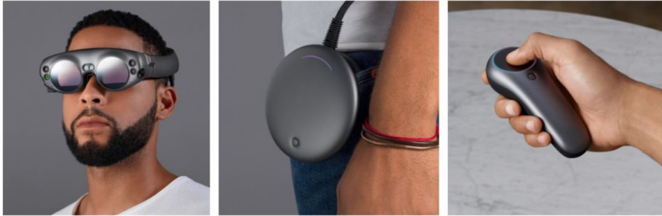
Figure 2.3: MLO hardware. From left to right: Lightwear, Lightpack and Control [6]
