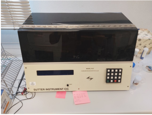
Figure 8: Puller used to pull sharpened micro-electrodes for the intracellular recordings.
