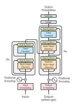
Figure 3.1: Transformer network architecture. To the left the encoder, and to the right the decoder. [2]
