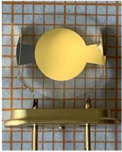
**Figure 67.** Typical QMB sensor used for chemical sensors and biosensors applications. QMBs are composed by a central quartz disc corresponding to the active surface area, held by a gold electrode pad. Credits: *Ref 214*.
