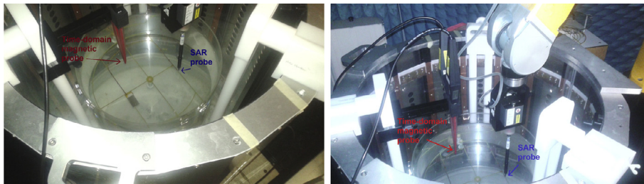
Fig. 6. Experimental measurement setup including the implant inside the birdcage coil resonator as well as one time-domain magnetic field probe and one SAR probe from two different perspectives. [6].
