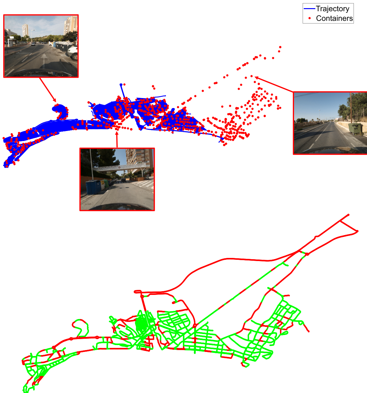
Fig. 1. Automatic container localization in the city of Benidorm, Spain. Top: Vehicle geo-positioned trajectory (in blue), human-annotated camera-captured containers (in red) and three examples of container appearances (surrounding blobs). Bottom: Automatically generated division between geo-positioned locations with (green) and without (red) containers for the proposed method. Note how the automatic localization of containers provided by the method highly correlates with human annotations. Furthermore, the method also proves to have high portability potential, as to avoid over-fitting to the target city, it was not trained using human annotations of this city but from ten other Spanish cities.
