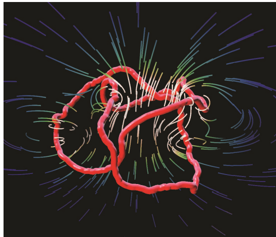
(B) Reconstruction of the vortex core and flow field from raw 3D data for the trefoil knot, [KI13; KSI14].
