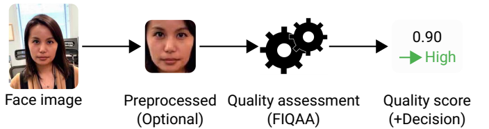
Fig. 1. Typical FIQA (Face Image Quality Assessment) process: A face image is preprocessed and a FIQAA (FIQA Algorithm) is applied, resulting in a scalar quality score output, based on which a decision can be made. Face image taken from [67].
