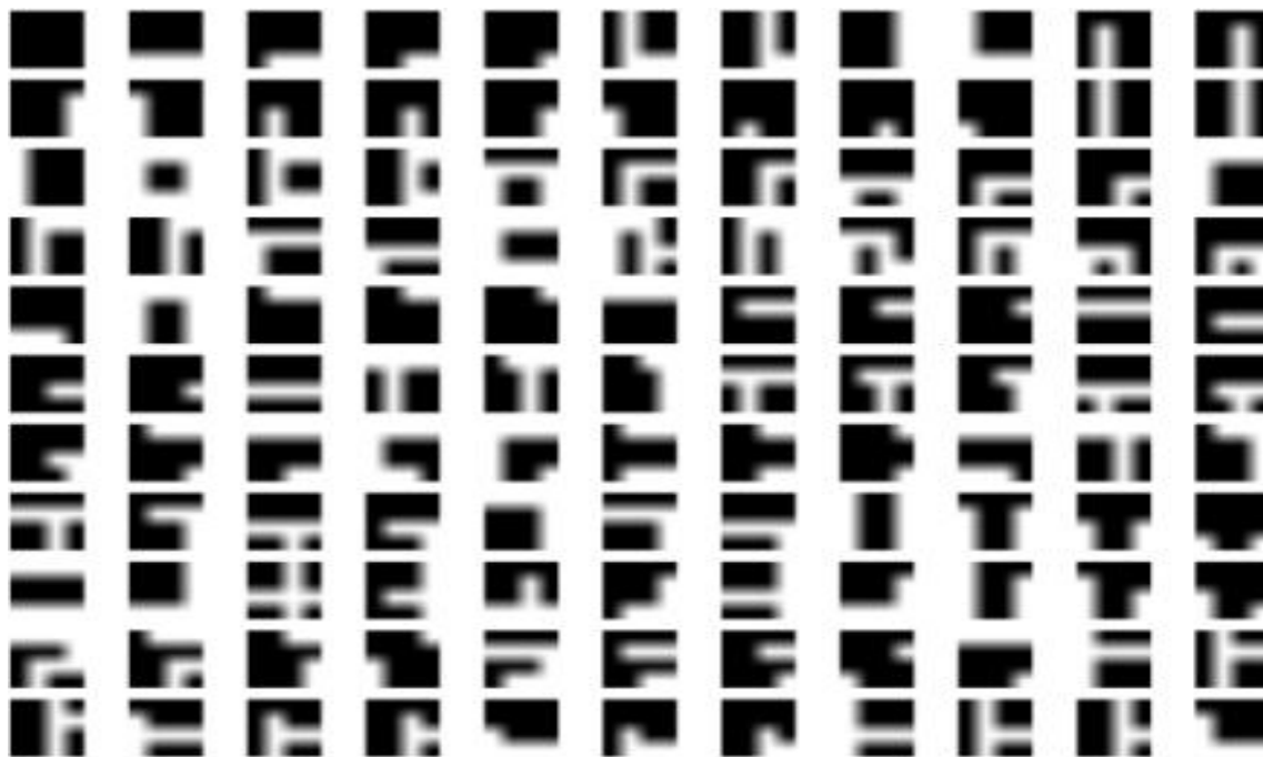
Figure 6.7: Spatial pooler quantization points. Quantization points stored by a node in layer 1 of the HTM image recognition system. Patterns correspond to parts of images over a 4x4 receptive field.
