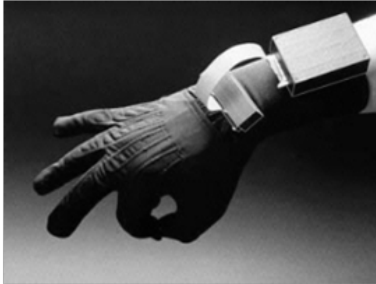
Figure 5.1: Electronic Data Glove. A glove similar to the one used to capture the sign language instances used in the Results part of this thesis. The glove provides dynamically data about the spatial position of the hand, the roll, pitch and yaw rotation angles of the wrist and the degree of bendiness of each finger.
