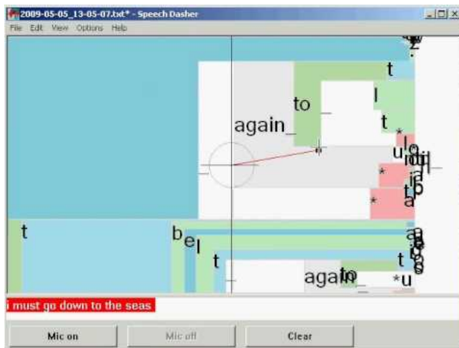
Figure 5.5: Gaze typing with Dasher. Letter selection is done by gazing at the incoming letters from the right. Letter size is correlated to its likelihood to follow the text written so far.
